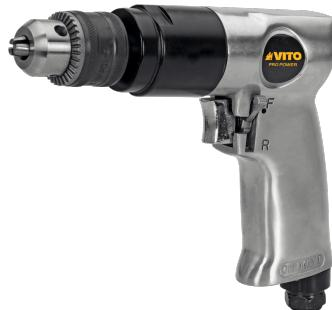
Pneumatic drill with an idle speed of 1800rpm, with a maximum air pressure of 6.2 bar, has an air consumption of 142L / min, with a maximum drill diameter of 10mm (3/8 ``), has a 1/4 `` air inlet connection thread, helping you to carry out your activities.
